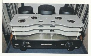
Looking fabulous in a gunmetal hue, with the company's signature wooden side sections, Auris' Fortissimo is a 100W/ch integrated amp operable in pentode or ultralinear modes, with power from four KT120s. Three line inputs plus one XLR and dimensions of 490x335x447mm (whd). www.aurisaudio.rs
