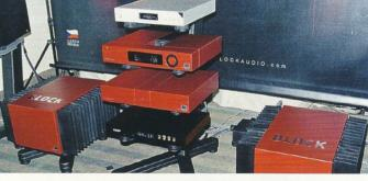
Block Audio showed its Line & Power Block dual-mono preamp with battery power supply, with 15 hours' operating time, driving the Mono Block 'Class A' mono power amps. The preamp offers single-ended and balanced inputs, and the user can select battery or AC operation. www.blockaudio.com
