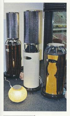
I got a whiff of Gravelli's amazing work on a plinth for E.A.T. at the Munich High End show. The company uses a damped polymer concrete material for a non-resonant enclosure in the digital-ready, active, 15kg, 160x380x280mm Virtuoso speaker. www.audio.gravelli.com
