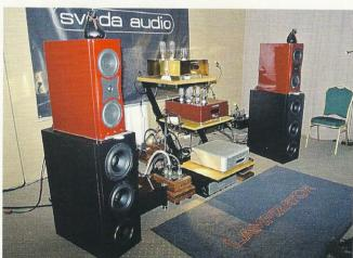
Polish high-end brand Lampizator demonstrated its Pacific Balanced DAC, and 211 Balanced monoblock amp it says produces 60W. Valves are two directly-heated 211 triodes, two 6H6P dual triodes and E88CC input tubes, with the Silk AC Filter just visible under the rack. www.lampizator.eu
