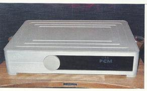
Hailing from Greece, Ideon's Absolute Hyperstream DSD/ DXD DAC is based around the popular ESS9038 Pro converter - its quad-channel architecture supporting balanced and singleended outputs and both USB and S/PDIF inputs. Two large linear PSUs are specified with custom transformers and seven stages of local regulation. www.ideonaudio.com
