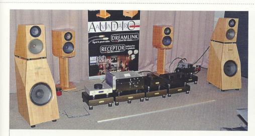
Seen in handsome bamboo woods, the Holophony Number 1 floorstanders and Number 4 standmounts from both ends of the four-model lineup are notable for high sensitivity. The former is said to be 97dB/1W, the small two-way 90dB. The Polish speaker builder favours paper cones and, apparently, employs 'original drivers from the '50s and '60s'. www.avatar-audio.com
