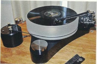
An oldie but a goodie, Scheu's Drive No 2, fitted with an SME 309 arm, can actually handle three tonearms. Design is clean and minimalist, with mass applied judiciously - the total weight is circa 38kg with the acrylic platter weighing 7.5kg. The three-legged chassis consists of a multi-layer glued acrylic frame with stainless steel base and is available in black or satin. Armboards are offered in acrylic, brass or bronze. www.scheu-analog.de
