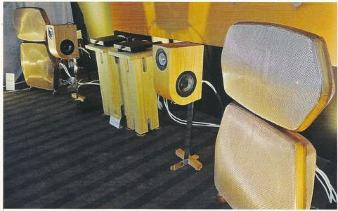
Among the more outlandish speaker makers at the show, Sound Kaos's collection includes the 1020mm-tall, copper-grilled Libération, which looks like a Quad '57 made by aliens. The open-baffle design houses an 18in woofer in the lower enclosure and a Raal ribbon super tweeter flanked by two 8in drivers up top. www.soundkaos.audio
