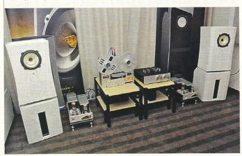
Two speakers from the vast range produced by Acoustique Quality from the Czech Republic - the catalogue runs to 32 pages. The radical, angular Passion Orca to the left is brand new, the company remaining tight-lipped about its specs, but the Passion Teen on the right is a two-way system with ScanSpeak 1in tweeter and 6.5in woofer in a 450x226x360mm (hwd) cabinet with a front port. The internal wiring is AQ solid-core. www.ag.cz
